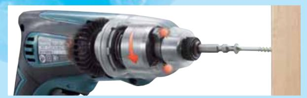
Finally, Hammer delivers enormous impact power onto Anvil, and the tool drives a screw with the high torque which rotational power alone cannot produce.
