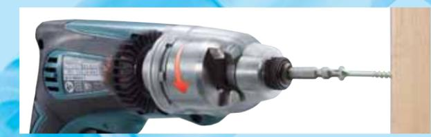
Hammer is now pulled closer to Motor, and finally the protruding portions of Hammer slip under Anvil, resulting in the release of tremendous energy which has been stored in Compression spring. And the released energy powerfully pushes and rotates Hammer.
